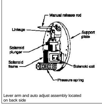
Figure 4-2. Support plate assembly
