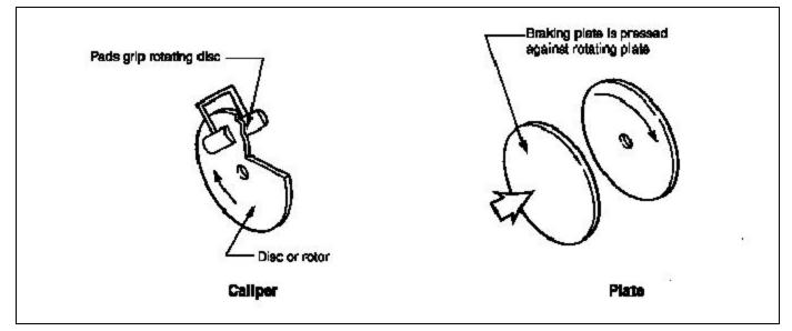
Figure 3-4. Typical disc brake types
