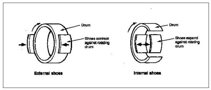
Figure 3-3. Typical shoe brakes
