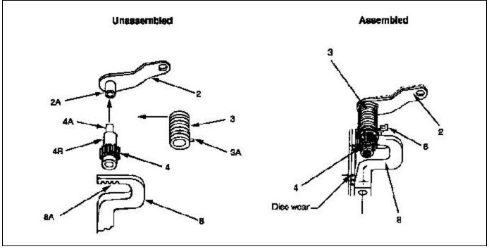
Figure 4-6. Operation of the self-adjusting mechanism
