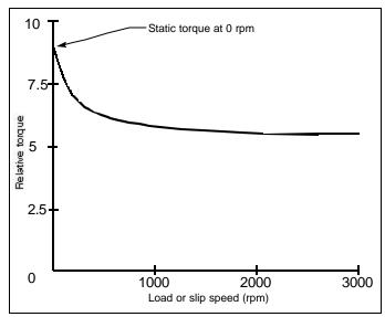
Figure 3-1. Friction brake torque characteristic showing static torque
