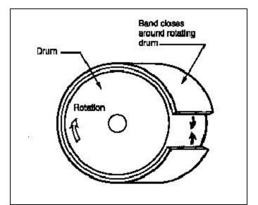
Figure 3-2. Typical band brake
