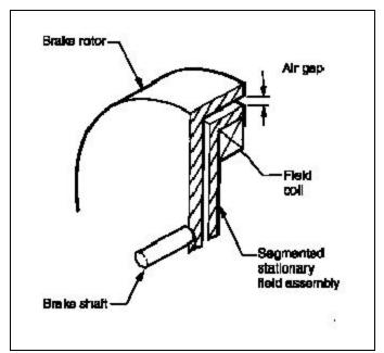
Figure 2-1. Typical eddy current brake
