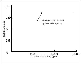
Figure 2-6. Typical magnetic particle brake torque characteristic
