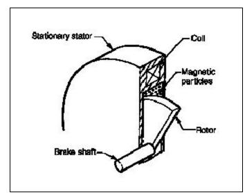
Figure 2-5. Typical magnetic particle brake
