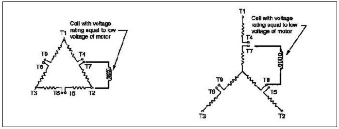
Figure 7-6. Connection to dual voltage motor
