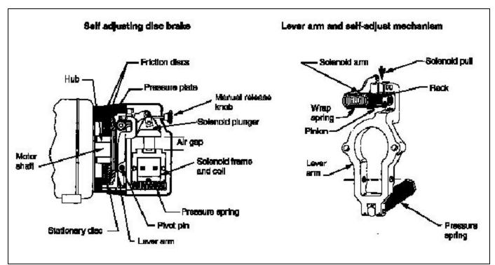
Figure 4-5. Typical Stearns self-adjusting disc brake mechanism
