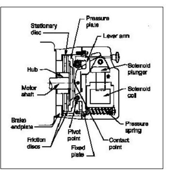
Figure 4-3. Brake in engaged mode
