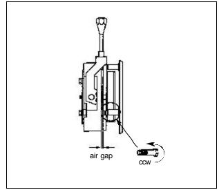
Figure 9-5. Wear adjustment- Adjustment bolts
