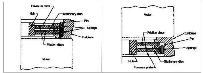
Figure 4-7. Vertical above modification, pins & springs
