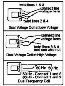
Figure 7-4. Dual voltage and Dual frequency coils
