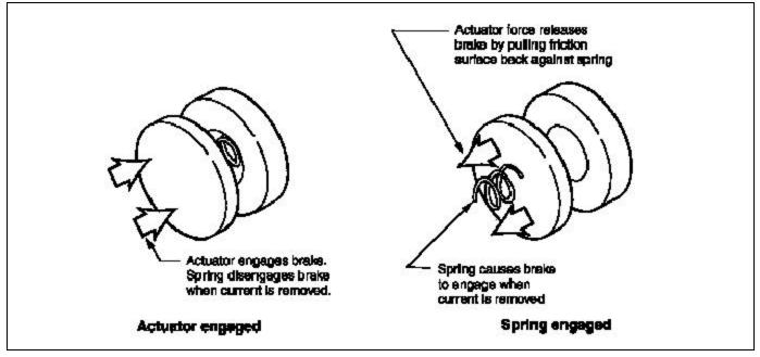
Figure 3-5. Two modes of friction brake operation
