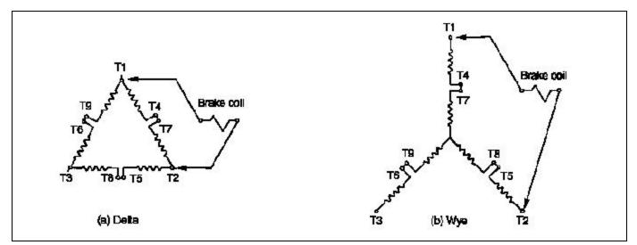
Figure 7-5. Connection to single-voltage motor
