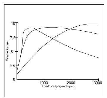
Figure 2-2. Torque characteristics for eddy current brakes
