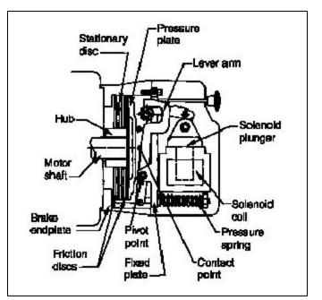
Figure 4-4. Brake in disengaged mode
