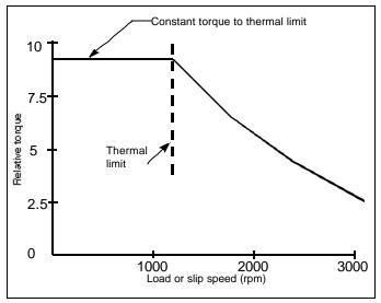
Figure 2-4. Typical torque characteristic for hysteresis brake
