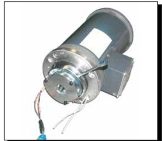
Quiet Brake Assembled to Motor
