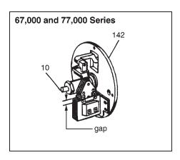
To replace the coil (12A), disconnect lead wire terminal screws (139S), lock washers (139W) and lead wires. It is not necessary to remove the support plate assembly (142).
