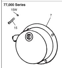
Remove four housing cap screws (15), lock washers (15W), and housing (7) by pulling back.
