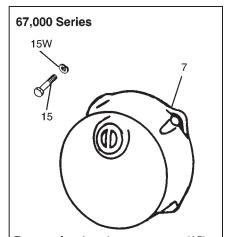
Remove four housing cap screws (15), lock washers (15W), and housing (7) by pulling back.
