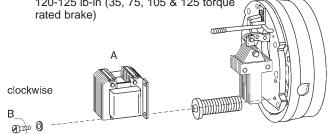
6 Reroute coil wires and reconnect to power supply.
